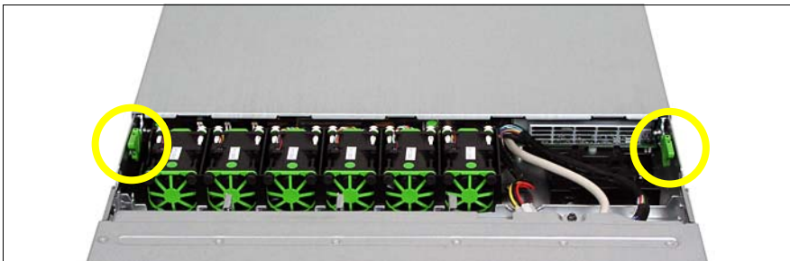
Figure 3: Removing the housing cover
